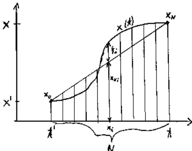
$$S[x(t)] = \int L(x(t)) dt = \int \frac{1}{2} m \left( \frac{x_i - x_{i-1}}{t_i - t_{i-1}} \right)^2 dt$$
